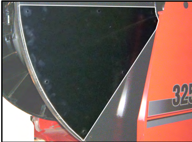
Figure 3 - Expose Access Panel
