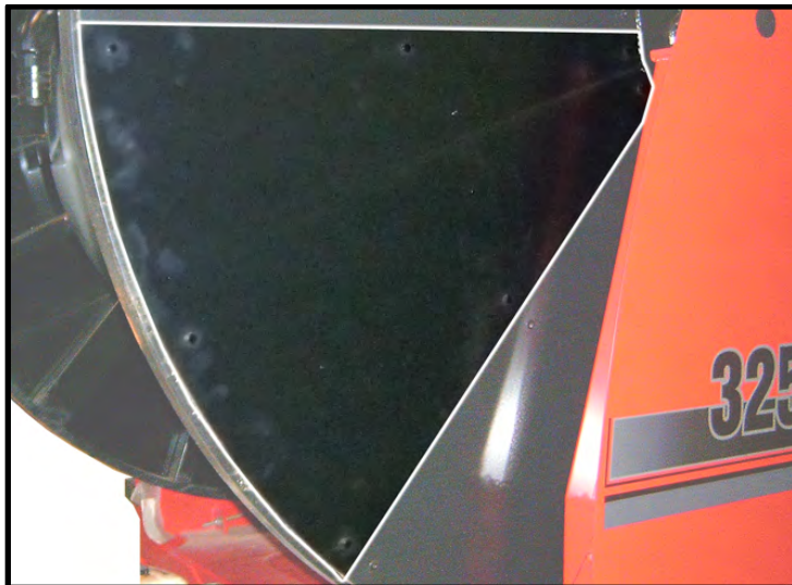
Figure 8 - Reinstall Access Panel
