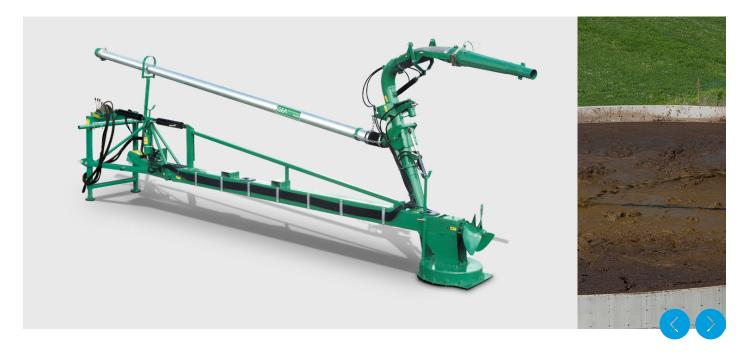
The Articulated Agi-Pompe stands out by its powerful propeller providing a constant agitation as you are in loading or agitation mode. This far-reaching pump allows faster agitation and transfer of manure from main storage. The Articulated Agi-Pompe rapidly homogenizes liquid manure using a tractor with a minimum of 140 HP – 540 RPM only. Also available in 1000 RPM with gearbox reduction.
