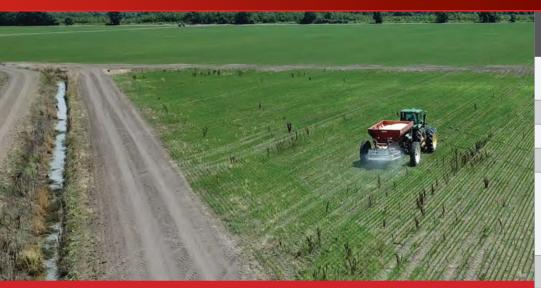
**Ideal for:** 120 foot dry fertilizer application with a high capacity single axle hopper for high speed application. 12 section spread pattern control to reduce overlap and application into environmentally sensitive areas.
