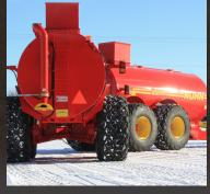
The Nuhn Quad Train, a multiple axle spreader, has gained popularity in the marketplace, both for its low maintenance and its reliability. The Nuhn Quad Train, with its unique and patented coupling system, is designed to perform as a single spreader. Its original design produces a tandem spreader capable of handling up to 15,000 gallons of manure that turns, backs up and handles more easily than a single large tank.
