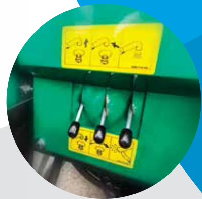
Hydraulic lever control
